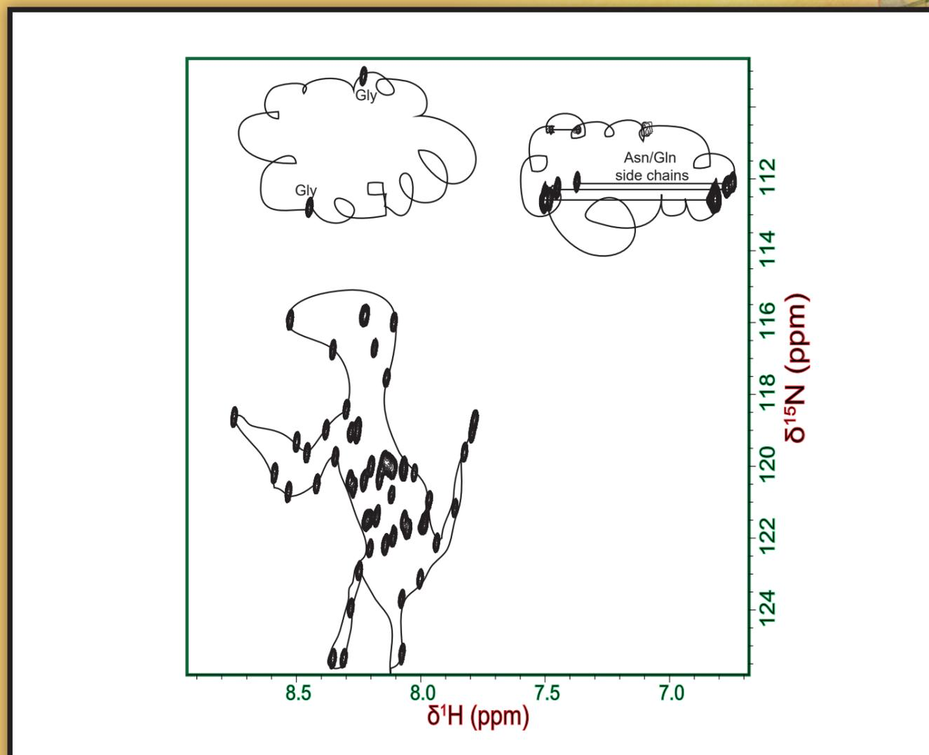
*2D  $[^{15}\text{N}-^1\text{H}]$  HSQC spectra of an intrinsically disordered protein recorded at pH 2.0 and 298 K on a Bruker Avance 800 MHz*
