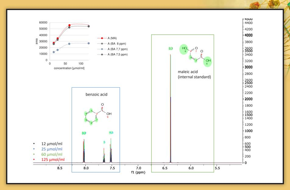
qNMR of benzoic acid with maleic acid as internal standard (in different concentrations)
