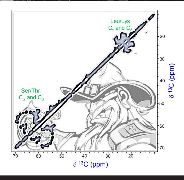
2D through-bond selective carbon-carbon correlation solid-state NMR spectrum of a 30 KDa human enzyme
