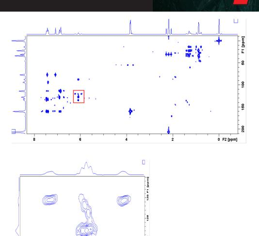
It is an organo-gold complex, containing one CF3 group. In our lab, we can record a 1D-19F spectrum at 400 MHz, but we can't record any 2D 13C-19F correlation spectra. We record therefore a 1H-13C HMBC and try to verify the CF3 group indirectly by its neighbouring CH2-group.
