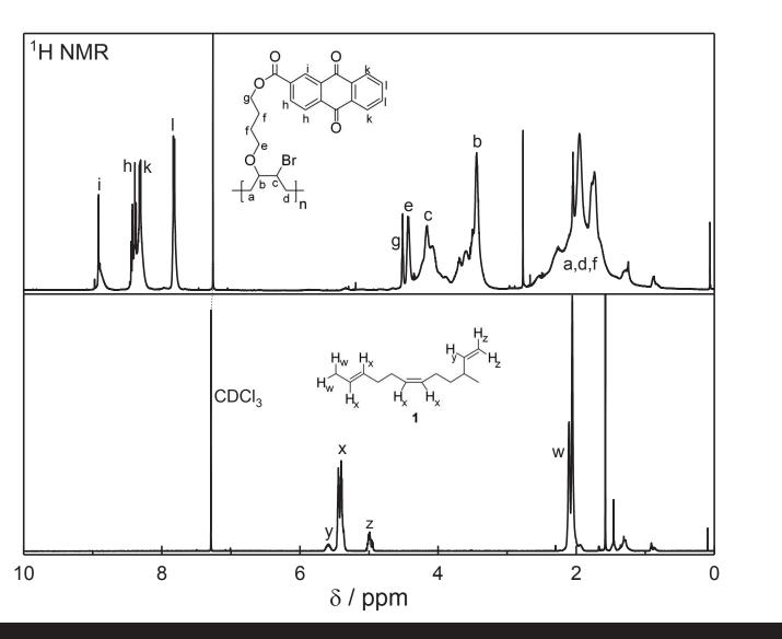
Postpolymerization-modified polybutadiene with anthraquinone carboxylic acid in CDCl<sub>3</sub>
