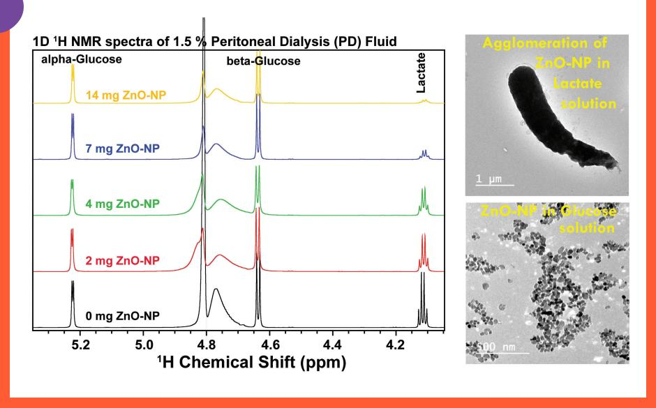
1D 1H NMR spectra of commercial peritoneal dialysis (PD) fluid in the presence of naked zinc-oxide nanoparticles
