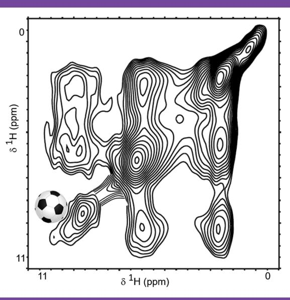
2D 1H/1H chemical shift correlation solid state NMR spectra of bone at 700 MHz under 42 kHz MAS with mixing time of 5 mins
