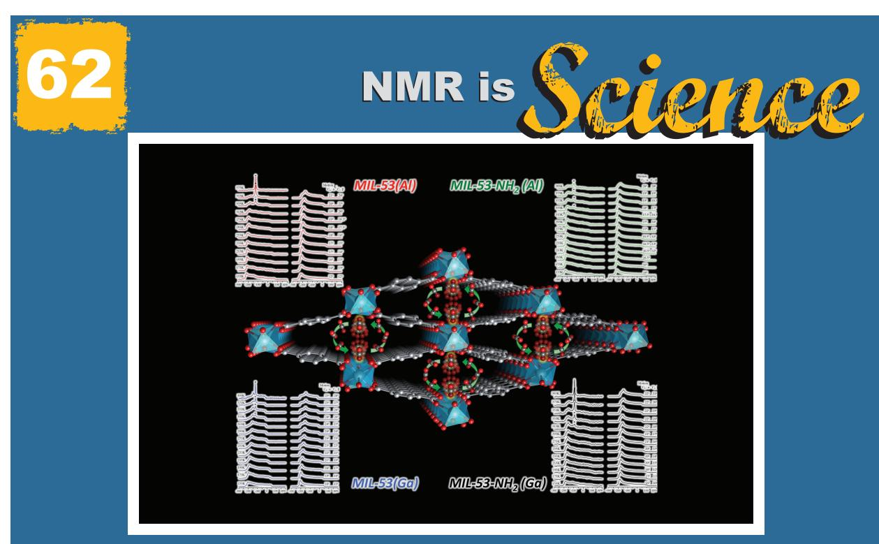
Static variable-temperature 13C solid-state NMR of dynamic carbon dioxide trapped in the MIL-53 metal organic framework
