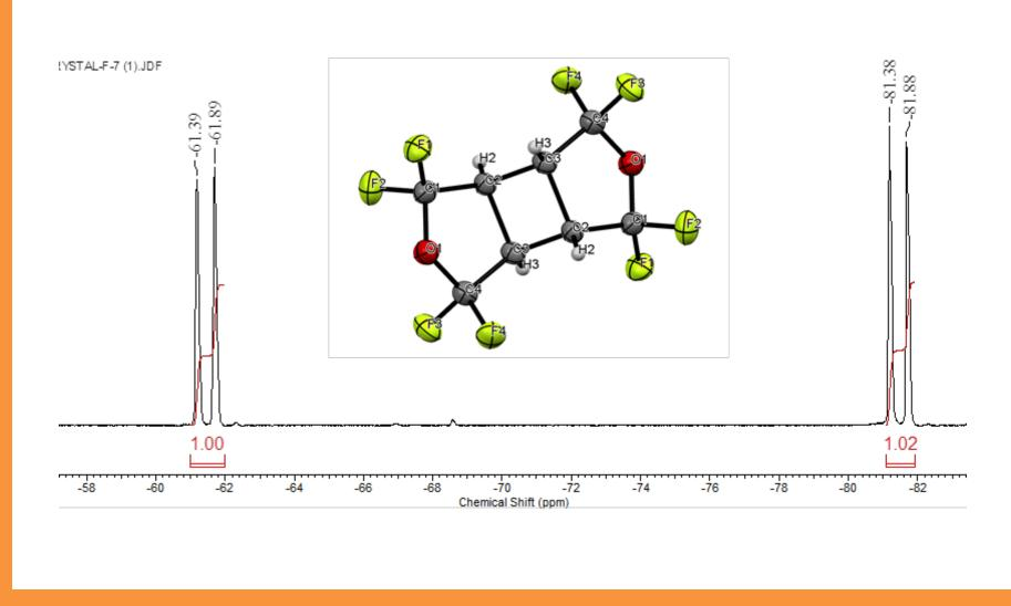
It is a cyclic dimer formed by 2,2,5,5-tetrafluoro-2,5-dihydrofuran under UV radiation. It has a chair-shaped conformation, and the four carbons in the middle are in the same plane with four hydrogen atoms pointing at opposite directions, which results in different chemical environment of the two fluorine atoms on each CF2 group giving an AB pattern in 19F NMR spectrum.
